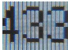
3MP LCD subpixel structure
